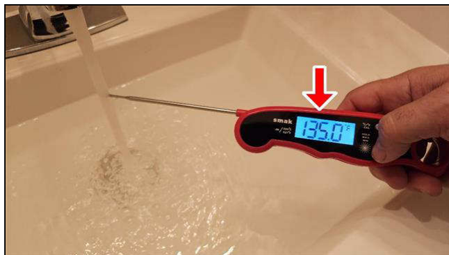
C. Item 2(Picture) downstairs bathroom sink (135.0 °F)
